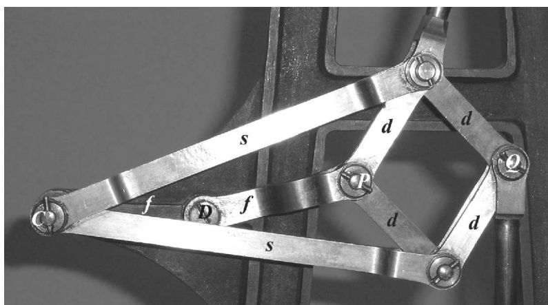
Figure 7. Working parts of the Peaucellier–Lipkin linkage.
