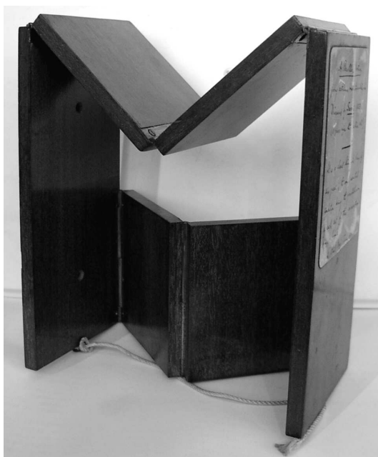
Figure 5. Sarrus Spatial Linkage for drawing a straight line. (Photo by Francis C. Moon, Cornell University, courtesy of the Cambridge University Engineering Department.)
